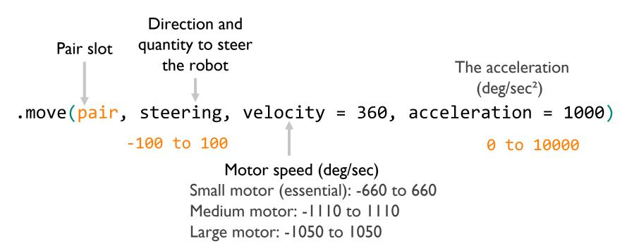
velocity=360 and acceleration=1000 are the default values if nothing is set. Positive steering values turn the robot right, negative turn left. Larger values turn more sharply, e.g., 0 moves straight, +/-50 moves one wheel only, +/-100 spins the robot.
