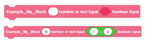
The blocks above are an example of a My Block with different inputs
